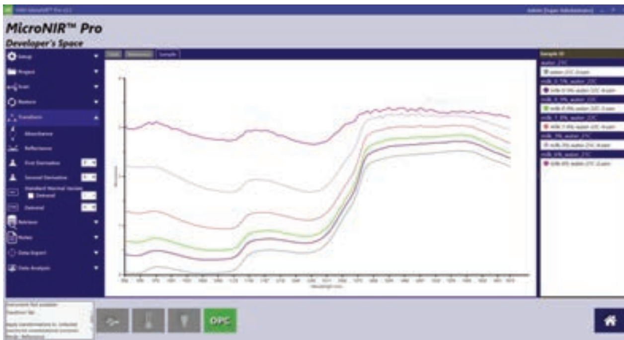
Figure 7. Spectra of whole milk diluted with water
