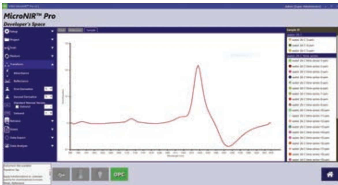
Figure 6. Water spectra acquired over 30 minutes with the 2 mm probe, indicating the absence of local heating
