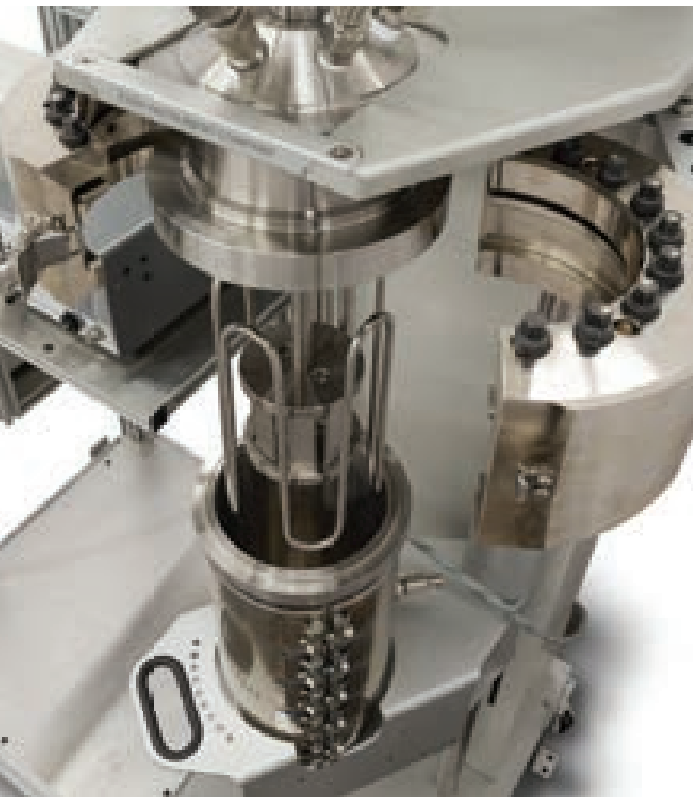
5 Liter Vessel lowered to reveal the rotating cage. In this configuration, up to 8 coupons at up to 2,000 rpm, can be tested at one time.
