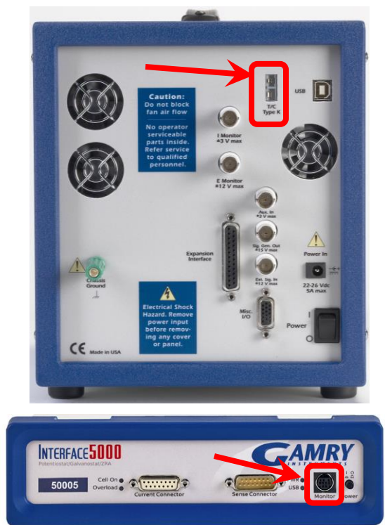
Fig. 3. Temperature-monitoring ports (circled in red) on the rear of the Reference 3000 (top) and front of the Interface 5000 (bottom) potentiostats.
